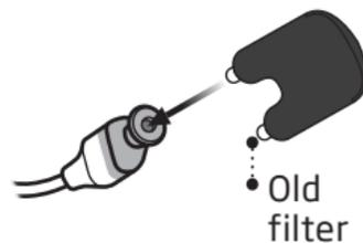
Insert the new wax filter using the other pin, remove the tool and throw it out.
