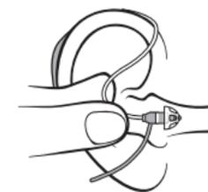
Hold the bend of the speaker wire between your thumb and index finger. The earpiece should point towards the ear canal opening.
