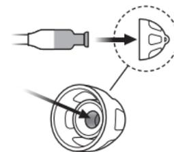
Insert the speaker exactly into the middle of the earpiece to obtain a firm attachment.
