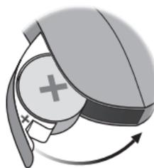
Close the battery drawer. The hearing aid will play a jingle through the earpiece. Hold the earpiece close to your ear to hear the jingle.
