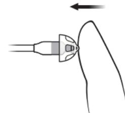
Push firmly to ensure that the earpiece is fastened securely.
