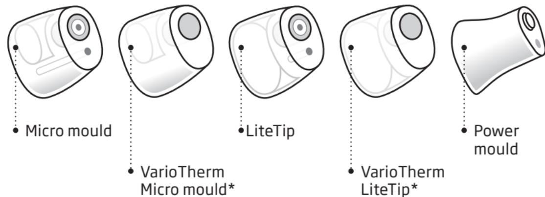
\* VarioTherm micro mould and LiteTip do not have wax filter
