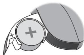
Insert the new battery into the battery drawer. Make sure the + side faces up.
