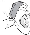
Gently pull your ear outwards and press the mould in the direction of the ear canal, twisting slightly.
