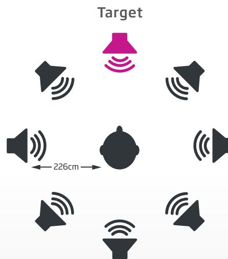
Figure 4. Spatial set-up of speech understanding task in noise and reverberation. Target presented at 0° and speech-shaped noise from surrounding loudspeakers.
