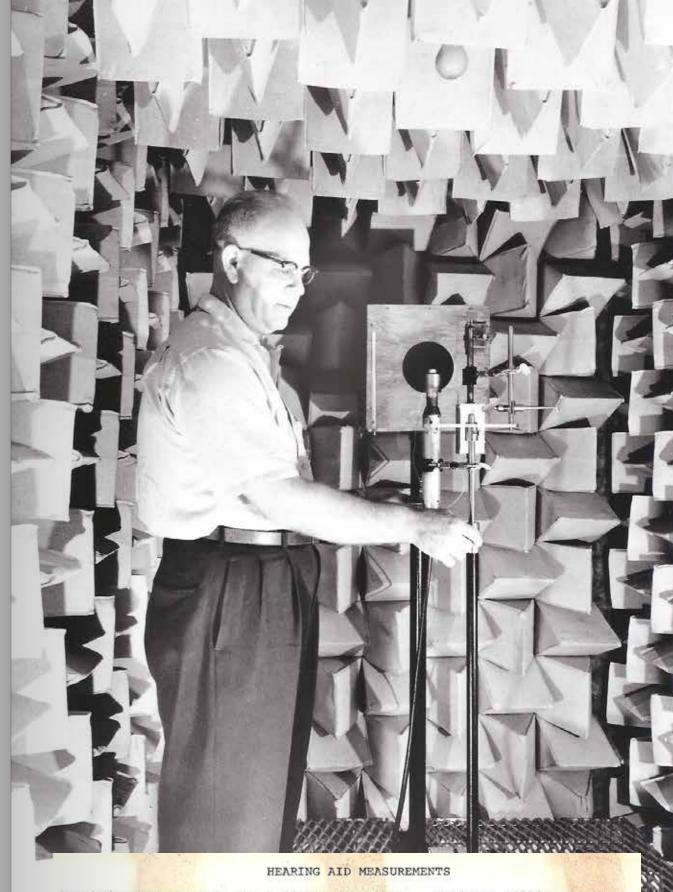
Anechoic Wedge Room in the Radioear Laboratory. Engineer William Steele is setting up a hearing aid to be tested in this room. The highly absorbent Fiberglas wedges "deaden" sound reflections that might otherwise make measurements inaccurate.
