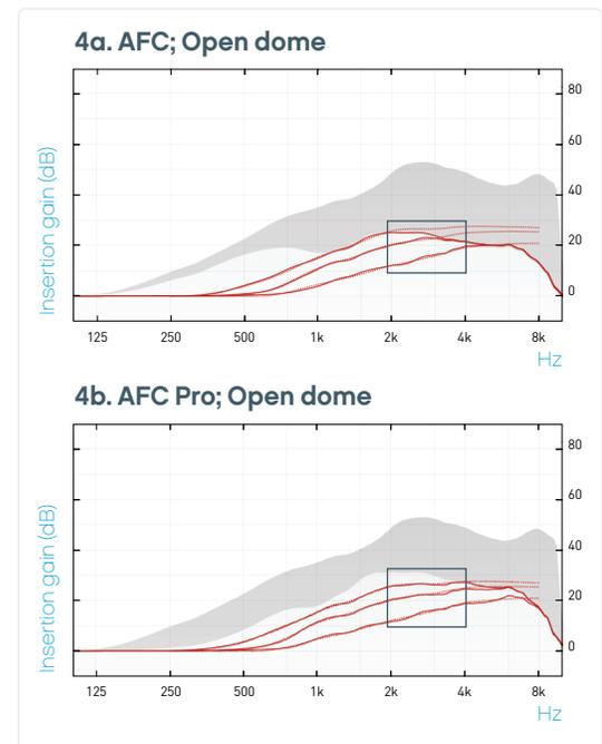
**Figure 4:** Feedback threshold margins for AFC (4a) and AFC Pro (4b) in EXPRESSfit Pro for open dome fitting. The feedback margin is lower for AFC and higher for AFC Pro.
