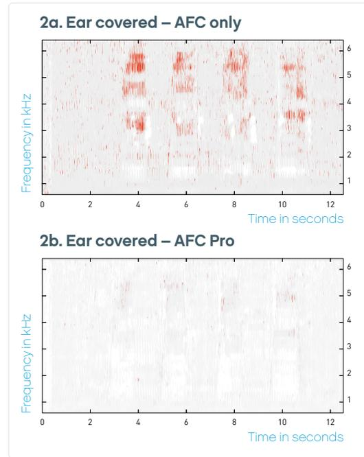
**Figure 2:** Spectrogram differences between hearing aid output with AFC (2a) and with AFC Pro (2b) as the device was covered and uncovered four times with a hand. The portions on the spectrogram representing acoustical feedback are shown in red. With AFC Pro, nearly all audible feedback has been eliminated from the output.
