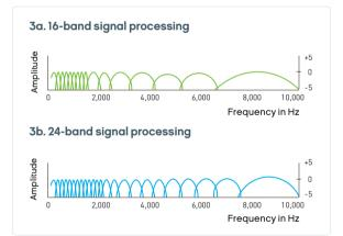
**Figure 3:** Frequency resolution based on 24 bands (3b) versus 16 bands (3a) allows more frequency-specific information from different signals i.e. noise and speech to be identified.
