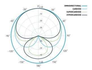
**Figure 2:** The directional characteristics of various microphone types in a free field. Using polar coordinates, the plots display along the radius how sensitive the various microphones are for sound approaching from all angles.
