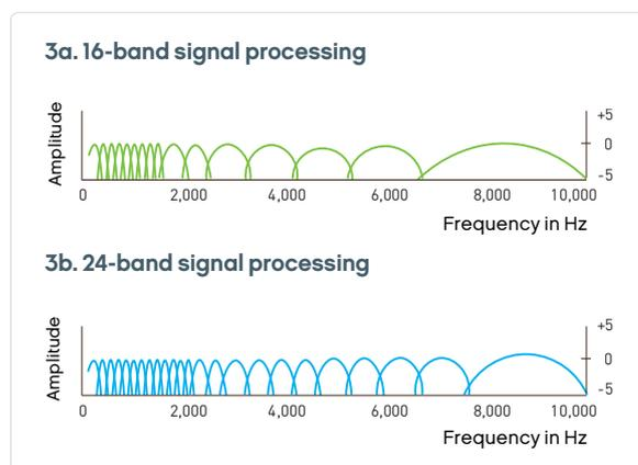
**Figure 3:** Frequency resolution based on 24 bands (3b) versus 16 bands (3a) allows more frequency-specific information from different signals i.e. noise and speech to be identified.
