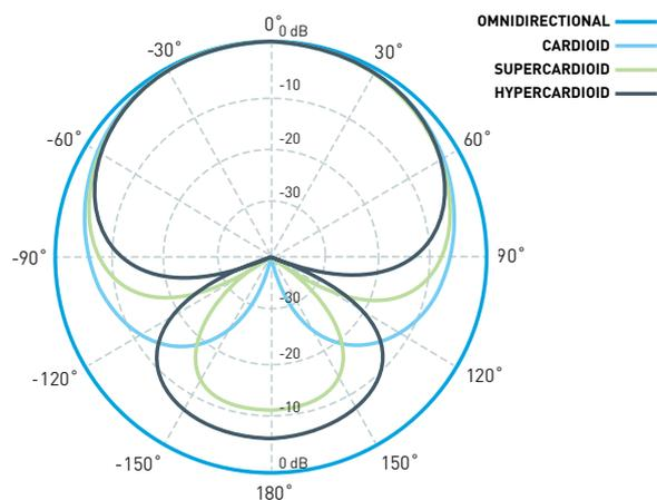
**Figure 2:** The directional characteristics of various microphone types in a free field. Using polar coordinates, the plots display along the radius how sensitive the various microphones are for sound approaching from all angles.
