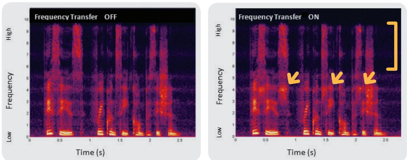
Figure 6: Spectrograms with Frequency Transfer off (left) versus on (right).
