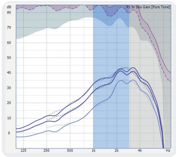
**1.0 – 2.9 kHz** When the suspected area of the cochlear dead region is extreme, the maximum Frequency Transfer shift occurs, from 1.0 – 2.9 kHz. Note: This range is only available on Super Power products.
