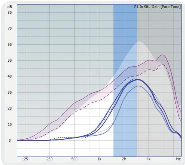
**1.5 – 2.9 kHz** When the suspected area of the cochlear dead region is very large, a strong Frequency Transfer shift occurs, from 1.5 – 2.9 kHz.
