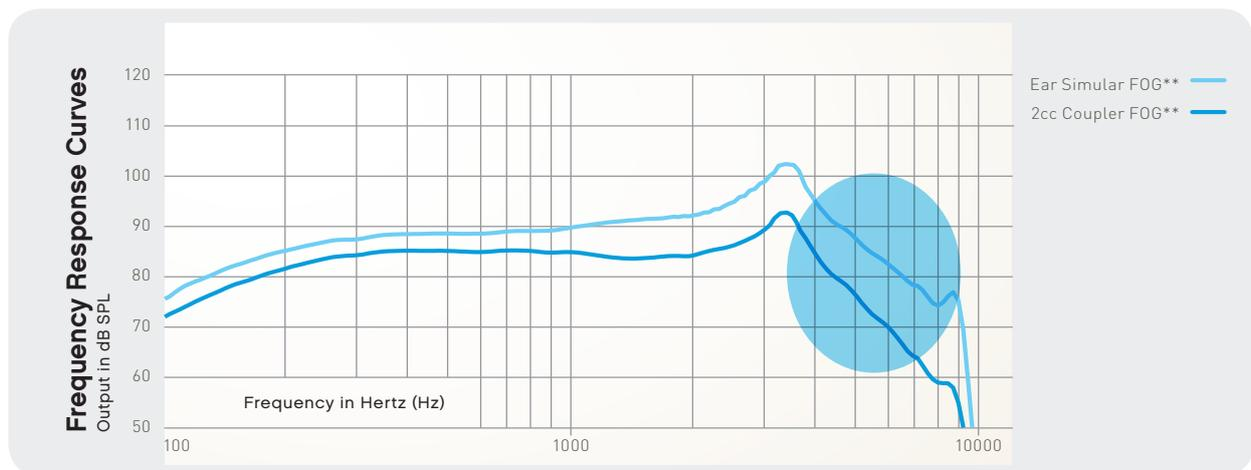
Figure 2: High-frequency roll-off typical of hearing instrument receivers.
