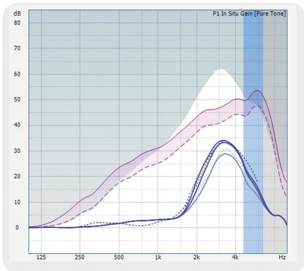
**4.6 – 6.5 kHz** When the suspected area of the cochlear dead region is small, a mild Frequency Transfer shift occurs, from 4.6 – 6.5 kHz.
