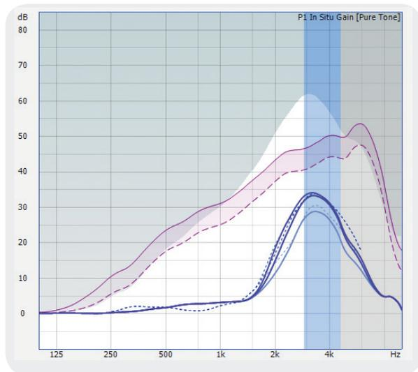
**2.9 – 4.6 kHz** When the suspected area of the cochlear dead region is larger, a moderate Frequency Transfer shift occurs, from 2.9 – 4.6 kHz.
