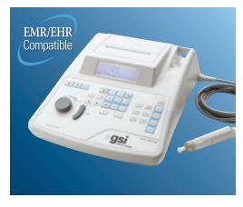
The GSI 39 Auto Tymp provides a flexible, screening product for tympanometry, acoustic reflex measurements and audiometry to meet testing needs today and in the future. The product is available in five different versions to meet the unique demands of each facility. All five versions are fast, versatile and easy to use. It is possible to add additional modalities such as audiometry, contralateral reflexes or 1,000 Hz probe tone as the facility testing requirements expand.
