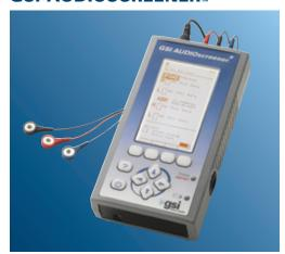
The GSI AUDIOscreener+ is a small, handheld hearing screener that is ideal for neonatal hearing screening programs, pediatrician offices and primary care physicians. Its universal display is easy to read and easy to use by non-hearing professionals. Choose OAE, ABR or OAE/ABR combination testing for a complete screening solution.
