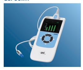
The GSI Corti is a portable, battery-operated diagnostic and screening instrument that measures Otoacoustic Emissions (OAE) for infants, children, and adults. The Corti offers maximum speed and flexibility with pre-defined and user-defined protocols for Distortion Product Otoacoustic Emissions (DPOAEs) and Transient Evoked Otoacoustic Emissions (TEOAEs) measurements.
